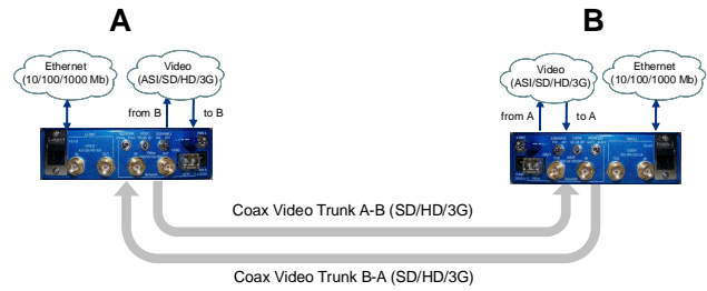
Figure 2: MSP-300 used for supporting two-way Video trunks/clients and Ethernet
