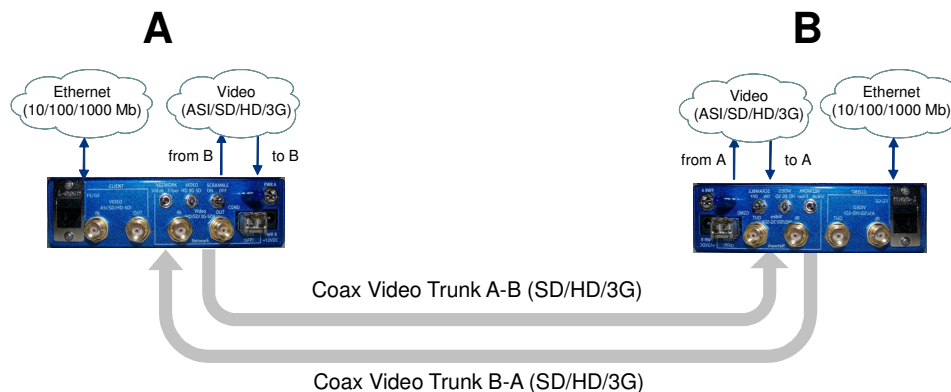
Figure 1: Carrying Ethernet over SDI Using MSP-300
